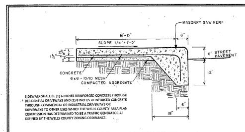
TYPICAL CROSS-SECTION VIEW STANDARD 6'-0" CONCRETE SIDEWALK & 6" CURB
